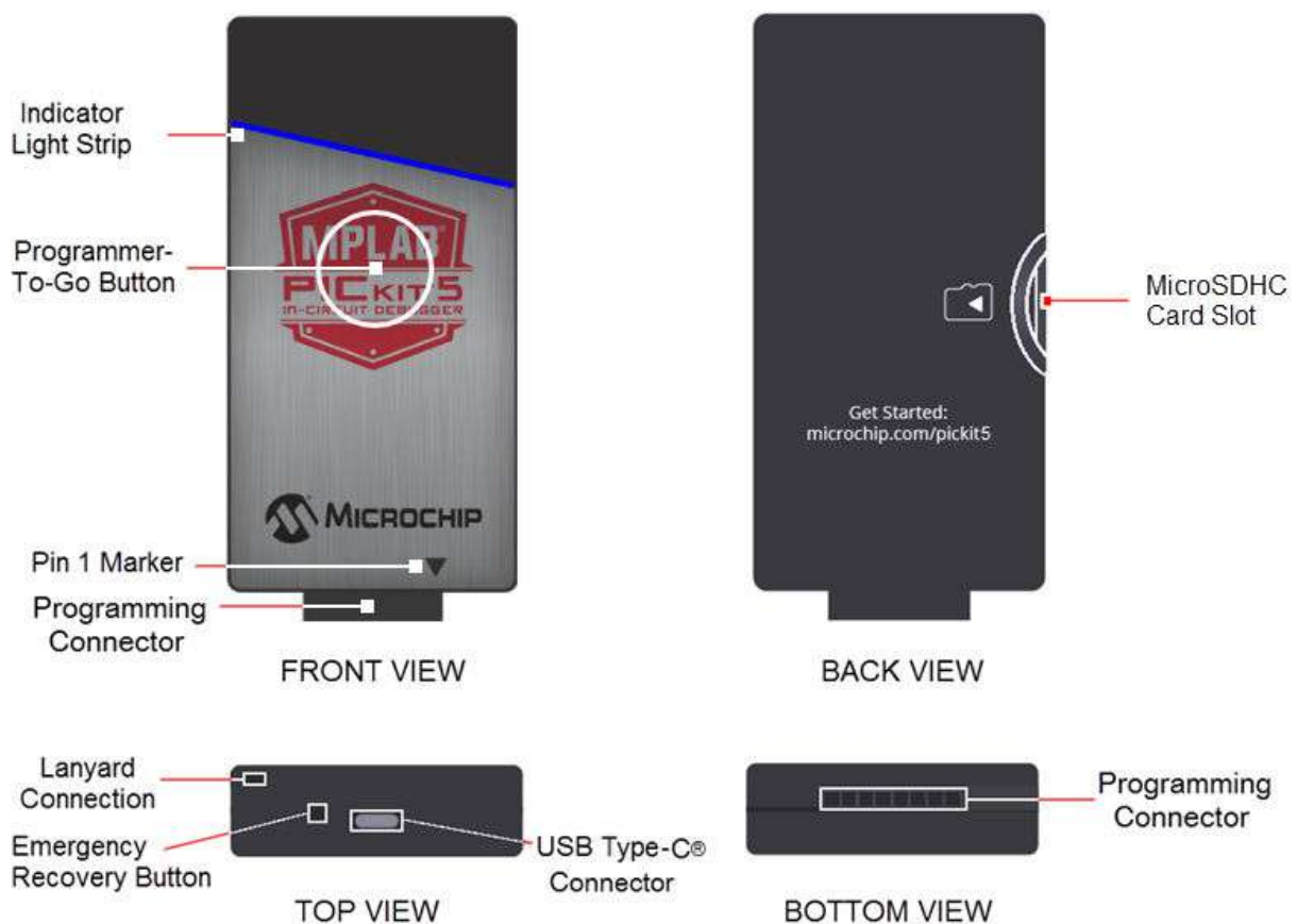
Figure 5-1. MPLAB® PICKit™ 5 In-Circuit Debugger Diagram
