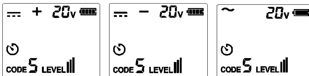
Figure 7.1.2b Voltage below 30V
