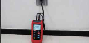
The locator can is used to find the correct RCD/GFCI or fuse location; No matter energized or none energized ones.
