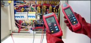
The measurement range is AC/DC 8~480V (AC frequency:50/60Hz), and the polarity can be identified.
