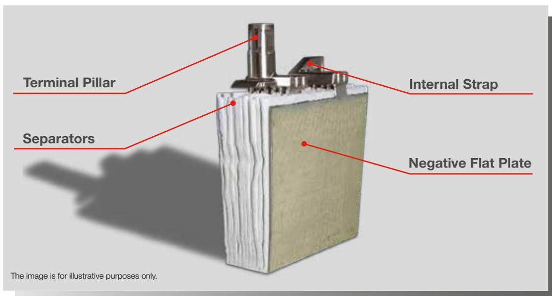
FIAMM SSLA RANGE USE AGM (ABSORBED GLASS MAT) TECHNOLOGY. THE ELECTROLYTE IS ABSORBED IN FIBERGLASS SEPARATORS WITH 99% INTERNAL GAS RECOMBINATION EFFICIENCY. BLOCS ARE GRANTS NON-SPILLABLE AND MAINTENANCE FREE THEREFORE REQUIRES NO TOPPING UP OF ELECTROLYTE DURING ITS WHOLE LIFE. LOW SELF-DISCHARGE ALLOWS 6 MONTHS SHELF LIFE.
