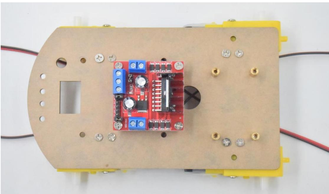
Note the direction of the motor driver board in the figure, after installation as shown above.
