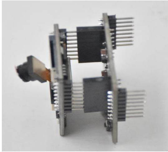
The ESP32 development board and ESP32-cam in accordance with the above map docking mode docking together
