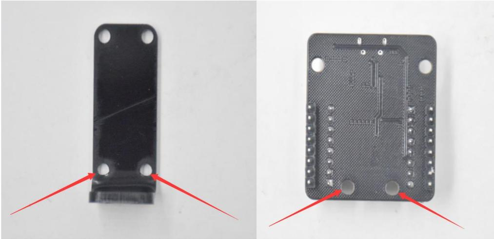
Locate the holes as shown above and use the M3X10 round head screw to secure the stand to the ESP32 Development Board.
