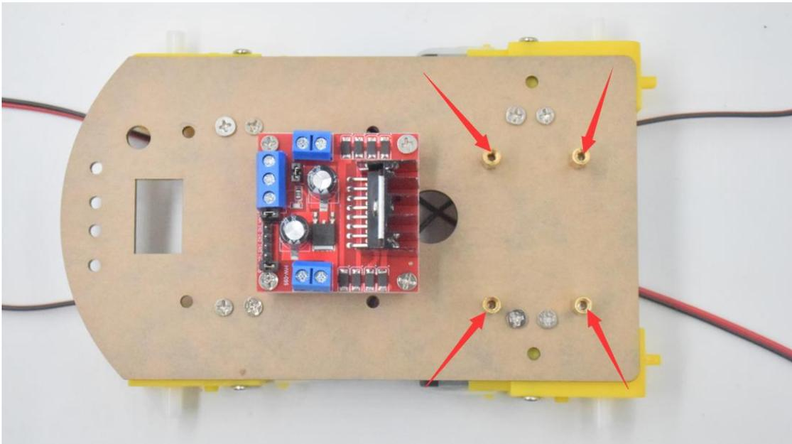
Find the 4 copper cylinder holes of the battery case as shown above, then open the cover of the battery case and fix the battery case with the M3X8 flat head screw. Note that the switch part of the battery case is facing up.
