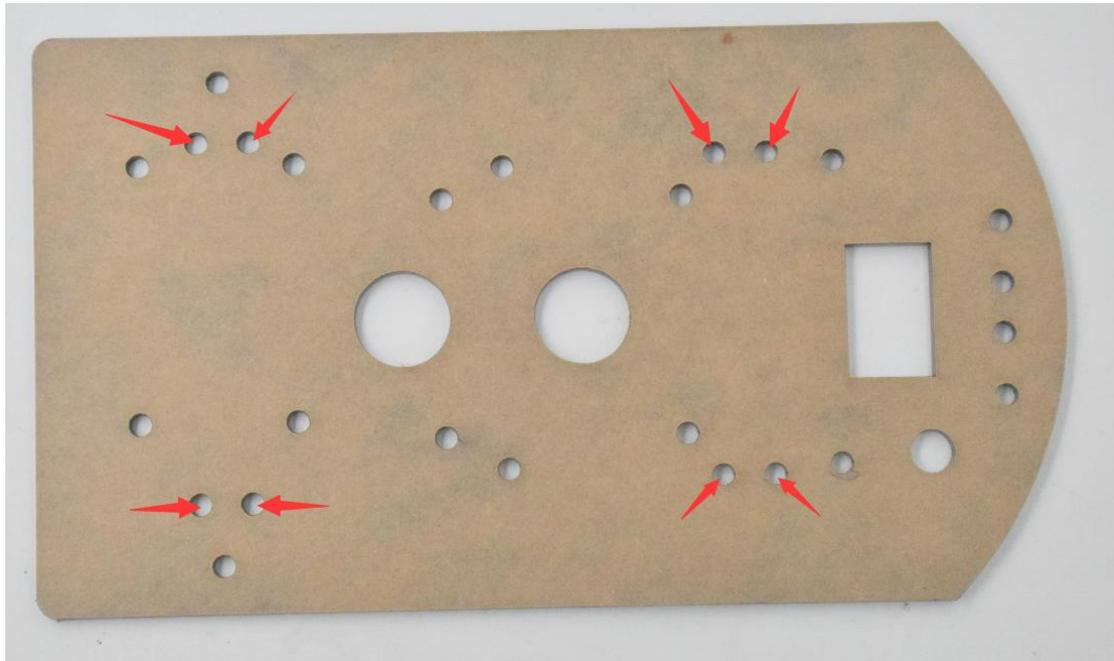
Use screws to secure the 4 motor brackets, as shown above.
