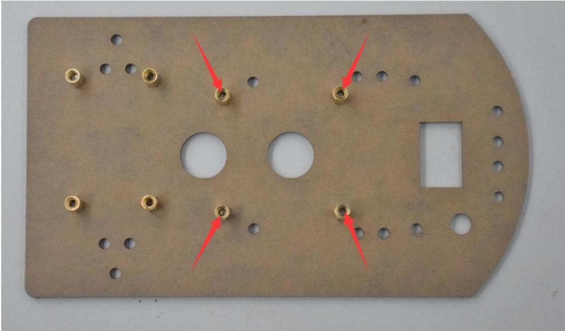
According to the above figure to find the corresponding 4 copper column position, the motor drive board with M3X8 screws fixed to the copper column.
