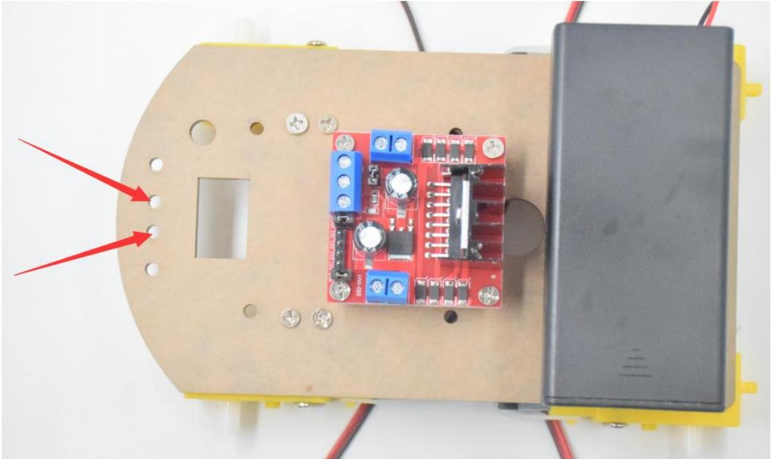
Use M3x10 round head screw to install the front assembled vertical bracket on the car bottom plate.
