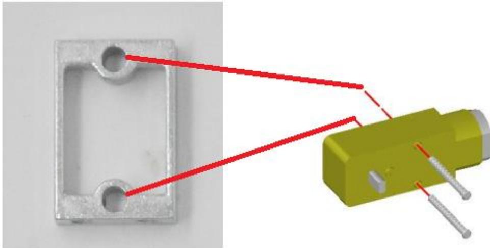
As shown above: use M3X30 screws to fix the motor to the motor bracket, then use the nut to tighten, when the motor is installed, pay attention to the electric melt glue part towards the red line of the internal motor upward, then the four motors are in turn fixed to the motor bracket.
