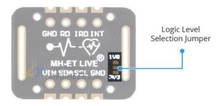
One of the most important features of the MAX30102 is its low power consumption: the MAX30102 consumes less than  $600\mu$ A during measurement. Also it is possible to put the MAX30102 in standby mode, where it consumes only 0.7 $\mu$ A. This low power consumption allows implementation in battery powered devices such as handsets, wearables or smart watches.
