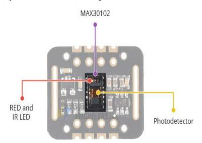
Behind the window on one side, the MAX30102 has two LEDs – a RED and an IR LED. On the other side is a very sensitive photodetector. The idea is that you shine a single LED at a time, detecting the amount of light shining back at the detector, and, based on the signature, you can measure blood oxygen level and heart rate.
