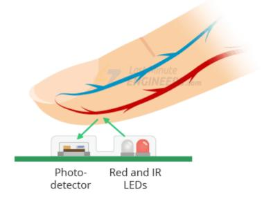
The MAX30102 works by shining both lights onto the finger or earlobe (or essentially anywhere where the skin isn't too thick, so both lights can easily penetrate the tissue) and
