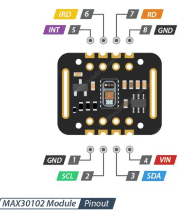
VIN is the power pin. You can connect it to 3.3V or 5V output from your Arduino.
