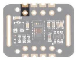
The INT line is an open-drain, so it is pulled HIGH by the onboard resistor. When an interrupt occurs the INT pin goes LOW and stays LOW until the interrupt is cleared.
