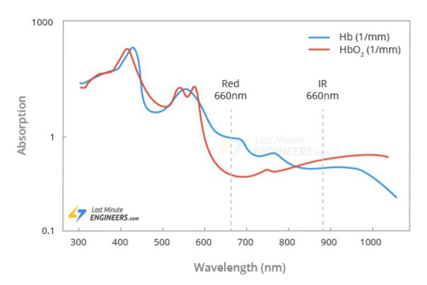
As you can see from the graph, deoxygenated blood absorbs more RED light (660nm), while oxygenated blood absorbs more IR light (880nm). By measuring the ratio of IR and RED light received by the photodetector, the oxygen level (SpO2) in the blood is calculated.
