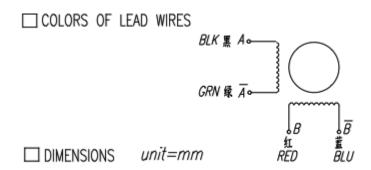
Coil wire diagram from the datasheet for NEMA-17 Stepper Motor.
