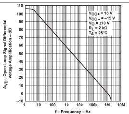
Figure 7. Open-Loop Large-Signal Differential Voltage Amplification vs Frequency
