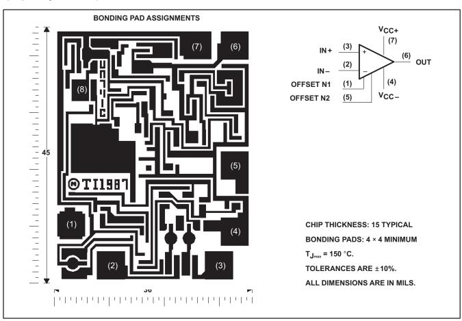
Figure 11. Bonding Pad Assignments
