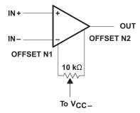
Figure 12. Input Offset Voltage Null Circuit
