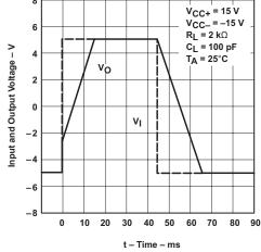
Figure 10. Voltage-Follower Large-Signal Pulse Response
