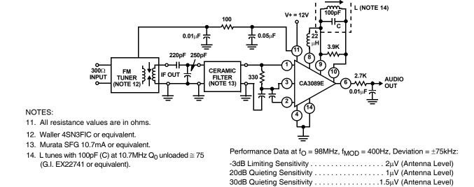
FIGURE 5. TYPICAL FM TUNER USING THE CA3089E WITH A SINGLE TUNED DETECTOR COIL
