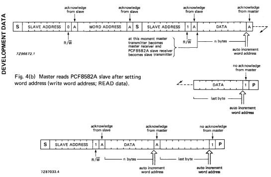
Fig. 4(c) Master reads PCF8582A slave immediately after first byte (READ mode).\*
