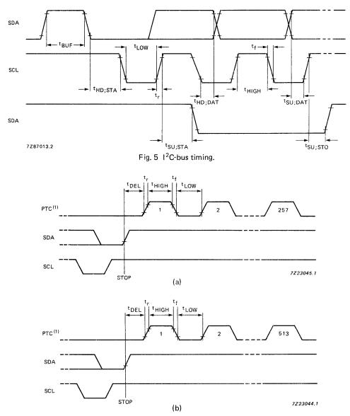
(1) If external clock for PTC is chosen, this information is latched internally by leaving pin 7 LOW after transmission of the eight bit of the word address (negative edge of SCL). The state of PTC then, may be previously undefined.
