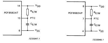
Figs. 3 (a) and (b) RC circuit connections to PCF8582AP and PCF8582AT when using the internal oscillator
