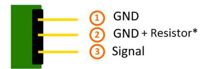
You can directly solder a resistor to the circuit board. In that case, the central pin (2), which includes the resistor, can be used.
