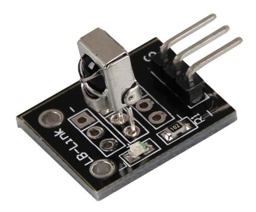
The KY-022 has three pins and responds to a carrier frequency of 38 kHz at 940nm. This signal is sent to the digital output. An LED module on the board will flash if an IR signal is detected.
