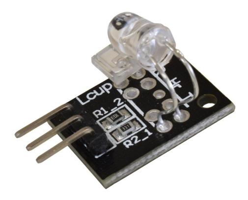
The KY-039 heartbeat sensor module can be used to detect the heartbeat signal using finger. This sensor has an analog output. By placing your finger on the module, you can see the heartbeat signal through the analog output pin.
