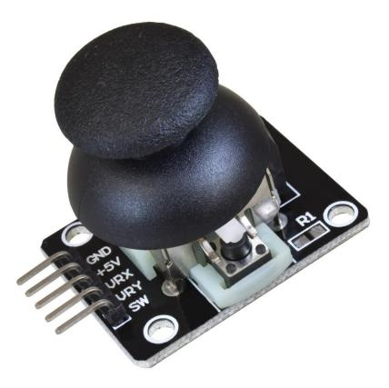
This Thumb Joystick is similar to the 'analog' joystick on PS2 (PlayStation 2) controllers. The X and Y axes are two 10k potentiometers which control 2D movement by generating analog signals. The joystick also has a push button that could be used for special applications.
