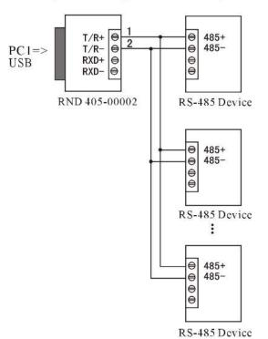
3.Half-duplex communication connection between RND 405-00002 interface converters
