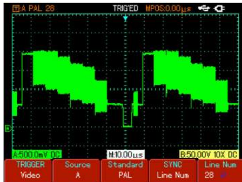
Figure 2-17 Video trigger : line synchronization
