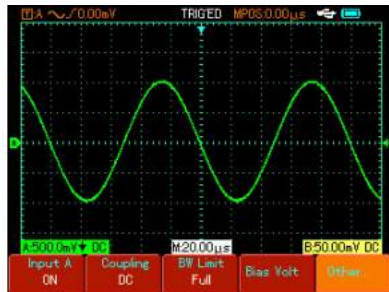
Figure 2-15 Channel polarity setup (inverted)
