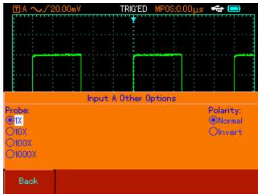
Figure 1-4 Adjusting the probe ratio
