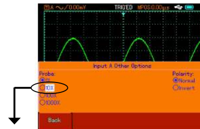
Figure 2-11 Setting the probe ratio
