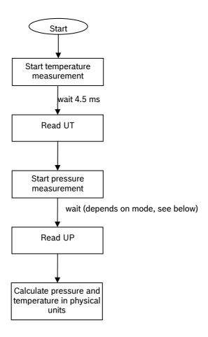
Figure 3: Measurement flow BMP180
