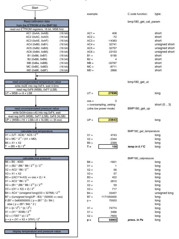
Figure 4: Algorithm for pressure and temperature measurement 销售热线:010-59457569 18001299538 陈先生
