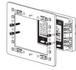
1 Place Head Unit behind panel, aligning mounting holes on panel with inner 4 holes (2 on each side of the unit). Attach with 4 (#6-32 x 1") Flat Head Machine Screws, threading into Head Unit brass inserts.
