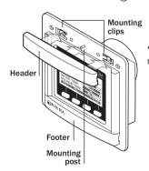
4 Snap header and footer into mounting clips and post.
