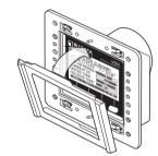
2 Place the 360 bezel onto the 360 panel with flat wedge up.
