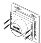
3 Fasten the bezel with 4 (#6-32 x 1.125") Flat Head Machine Screws through the back of the Head Unit and threading into the brass inserts in the back of the bezel.
