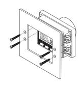
3 Place Head Unit flush through the back of the panel. Attach with 4 (#6-32 x 1") Flat Head Machine Screws through the panel, threading into the brass inserts in the Head Unit.
